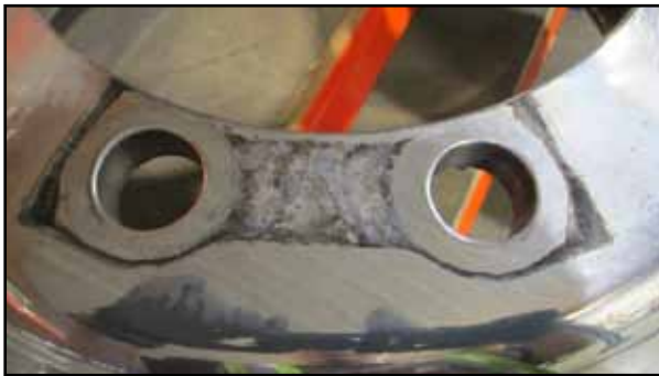
Galvanic corrosion mating faces wheel nut protection ring or cover
