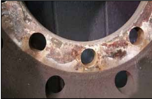
Galvanic corrosion at mating faces of wheel
