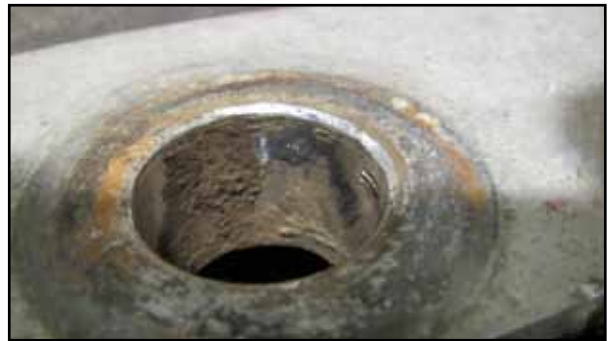
Galvanic corrosion wheel nut area
