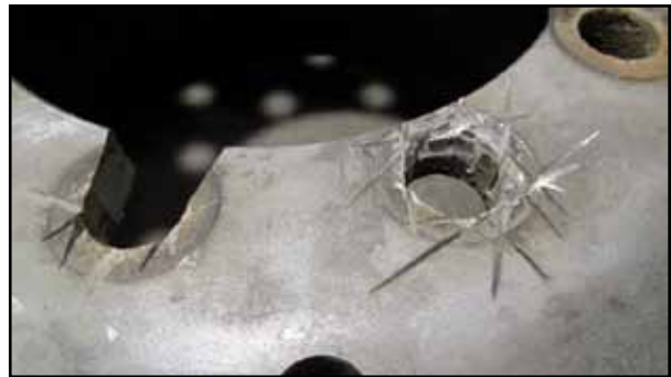
Wheel nuts needed to be cut out the wheel
